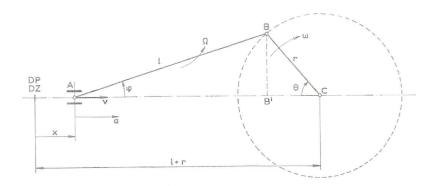
Figuur 1: crankshaft connecting rod mechanism
