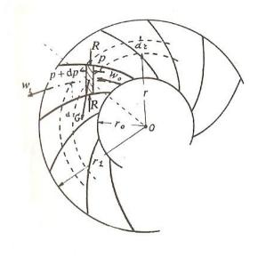
Figuur 2: forces on an amount of fluid in a fan
